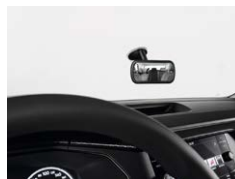
Inside rear-view mirror (Additional) - Suction cap mounting
