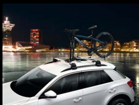
Bicycle holder 17kg, only in conjunction with: Roof bars and supporting rods with T groove profile
