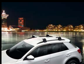
Supporting rods T-groove
