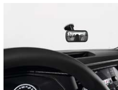
Inside rear-view mirror (Additional) - Suction cap mounting
