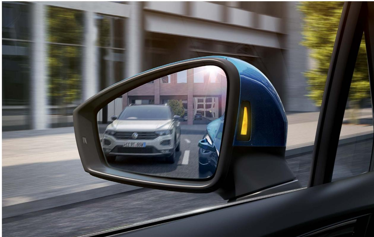
Through Lane Assist and Side Assist, the Touareg helps prevent potential collision using a camera-controlled warning system to monitor the vehicle's position in relation to road markings and other cars. Using the Head-up Display, the Touareg will alert you to any dangers while you keep your eye on the road.
